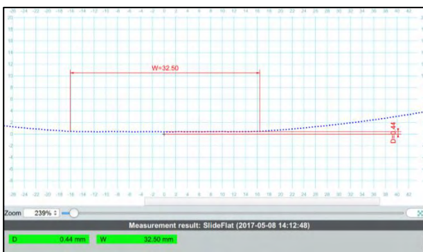
MEASUREMENT METHOD „SLIDFLAT“
