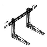
**6** Fit the anti-vibration blocks, adjust the rear adjustment wheels
