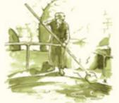
3 **Refining and pouring** After being washed several times, a perfectly neutral (0% alkalinity) paste is obtained. It is then poured directly onto the floor where it cools and hardens.
