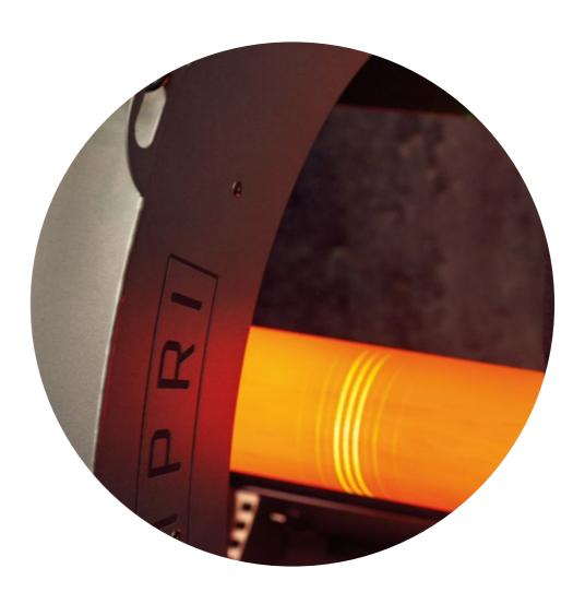
Forget about conventional approaches: In the future, you can evaluate the profile of your long goods directly, during hot rolling without the cooling phase, and continuously monitor dimensional accuracy and surface quality with just one test system. Our mobile profile measuring devices CALIPRI RCX and the stationary combined testing systems OSIRIS are equipped with the latest laser light section technology, in order to guarantee the highest accuracy.
