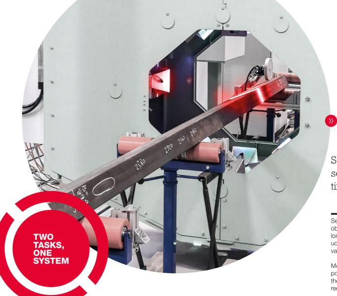
Sophisticated laser light section sensors detect the tiniest deviations.
